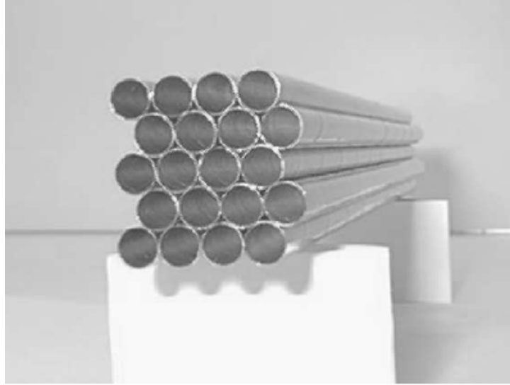
Figure 3.4: A close-packed array of 20 tubes bonded together [51].
