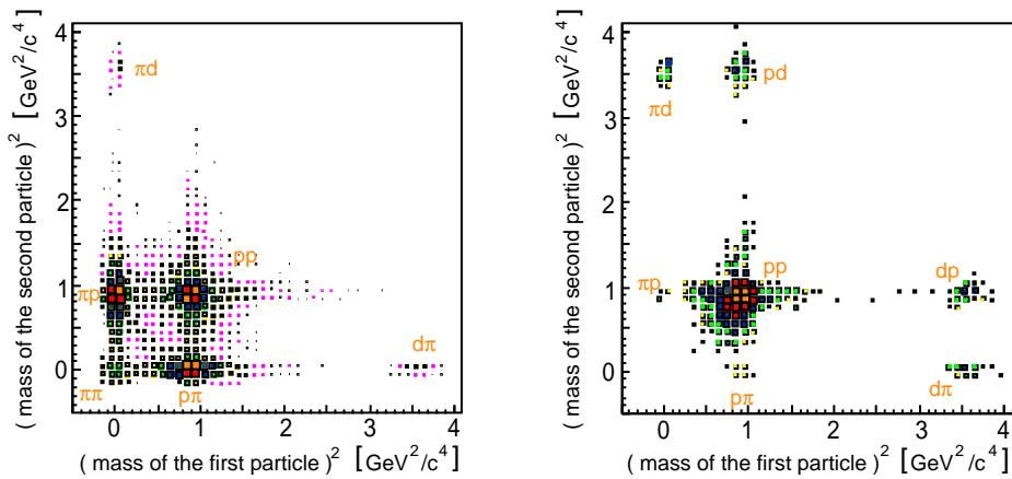
**Figure 3.1:** **Left:** Squared masses of two positively charged particles measured in coincidence in the  $pp \rightarrow A^+B^+X$  reaction. **Right:** Squared masses of two positively charged particles measured in coincidence in the  $dp \rightarrow A^+B^+X$  reaction. The size and colours of boxes correspond to the number of entries expressed in logarithmic scale.
