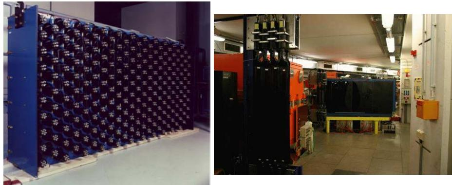
**Figure 2.9:** The COSY-11 large scintillator wall (S3, "AMADEUS") before installation (left: rear view) and at COSY-11 (right: front view).
