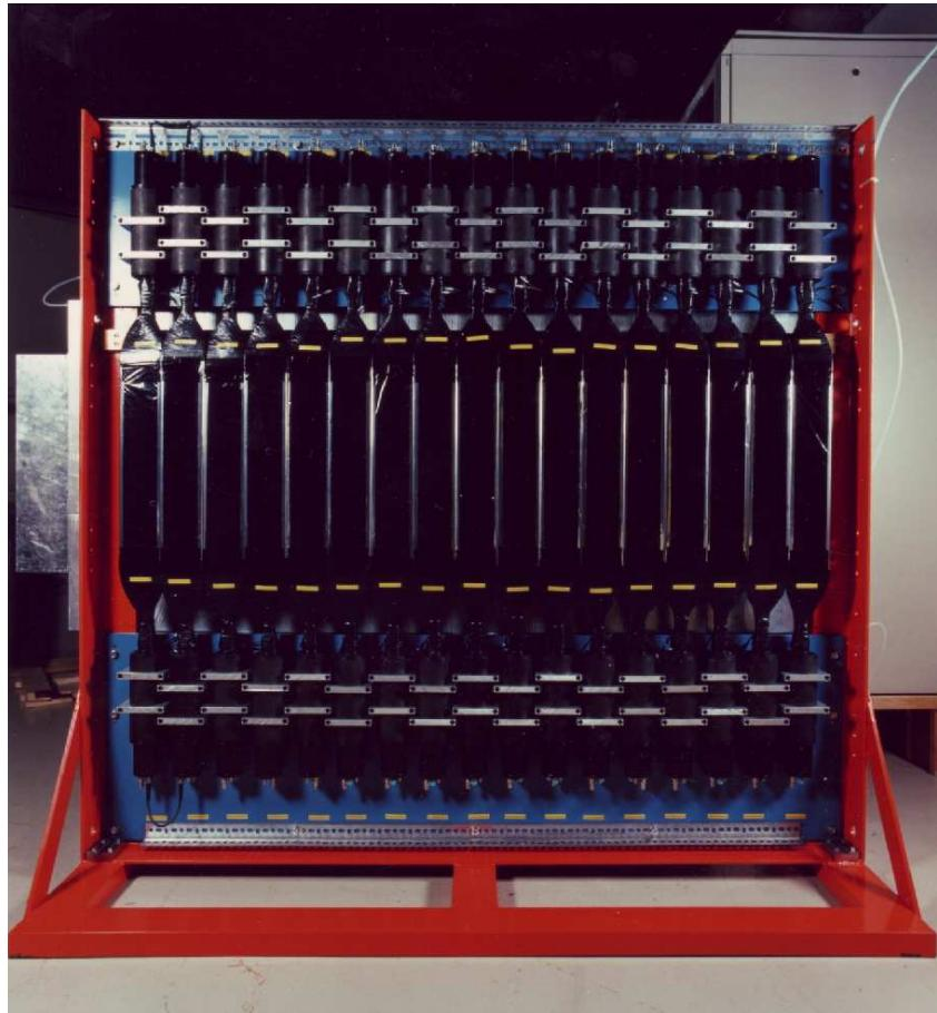
**Figure 2.8:** The COSY-11 hodoscope before installation consisting of 17 scintillator bars and readout on both sides.
