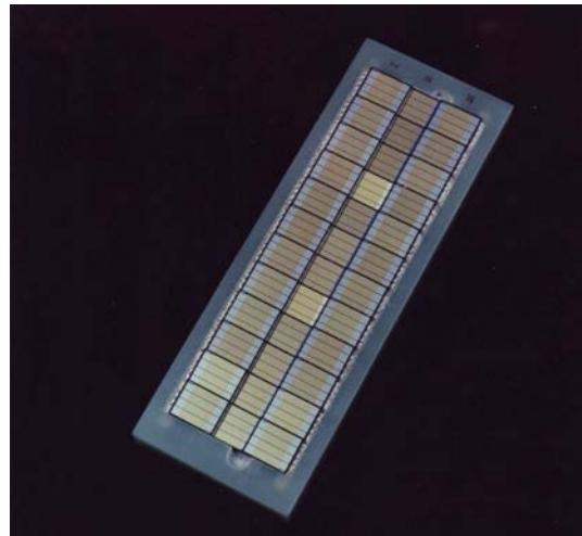
**Figure 2.10:** One module of the COSY-11 silicon pad detector consisting of 144 independent detection units.
