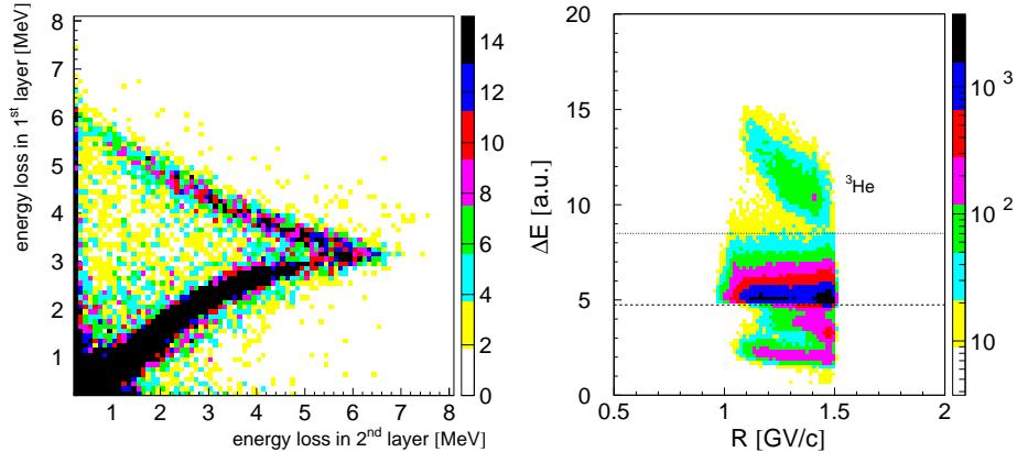
**Figure 3.3:** **Left:** Energy losses in the first versus the second layer of the silicon pad detector (spectator detector). The data were taken with a deuteron target and a proton beam with a momentum of 3.365 GeV/c. **Right:** Energy loss in the 4 mm thick plastic scintillator of the S1 hodoscope shown as a function of the magnetic rigidity. The lines indicate a hardware and software cut on the energy loss used in the analysis of the  $d\mu \rightarrow ^3\text{He}\eta$  reaction.
