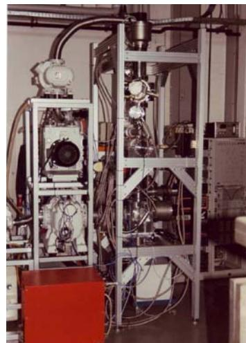
**Figure 2.4:** The arrangement of the cluster target before installation at COSY-11.
