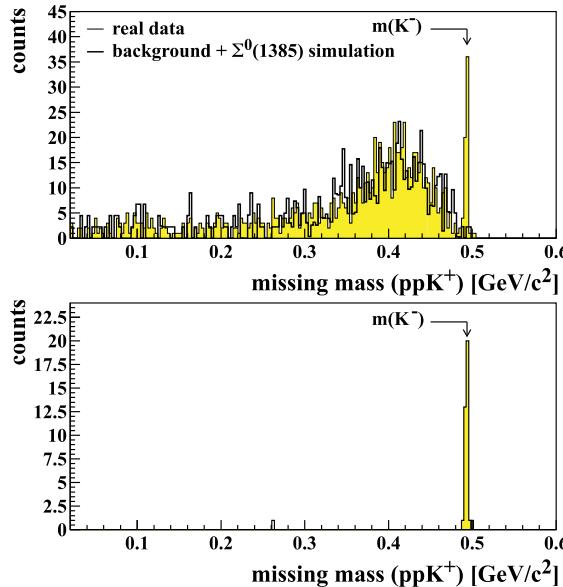
**Figure 3.7:** Missing mass distribution of the  $ppK^+$  system at an excess energy of 17 MeV above threshold. The picture on the top presents events with identified protons and  $K^+$  meson (thin solid line). The spectrum indicated by the thick solid line is a reproduction of the background distribution. The lower spectrum represents events with an additional hit in the silicon pad detector, at the position expected for the  $K^-$  meson.
