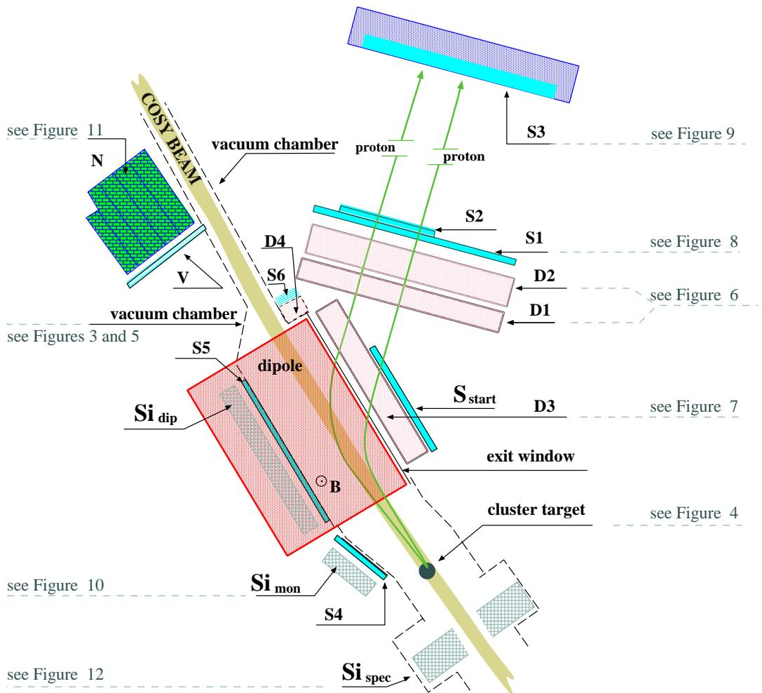
**Figure 2.1:** A drawing of the COSY-11 facility for close-to-threshold measurements
