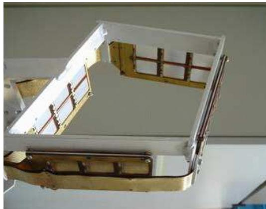
**Figure 2.12:** The array of Si-pad detectors surrounding the target region.
