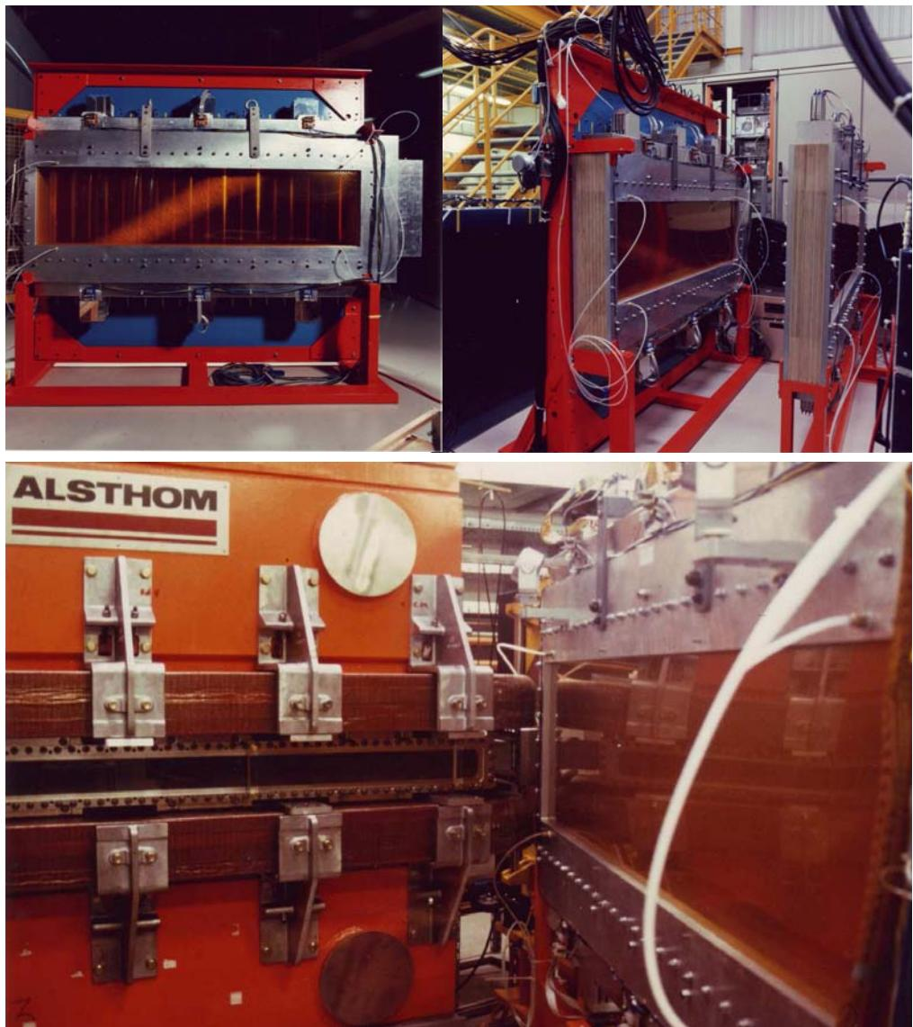
**Figure 2.6:** Three different views of the drift chambers, front and side view before installation (top), after installation next to the COSY dipole (bottom).
