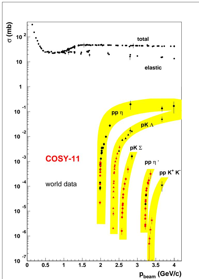
**Figure 1.2:** Proton–proton cross sections for different reactions of the light meson production in the threshold region. For comparison also the total and elastic cross sections of proton–proton scattering are shown.
