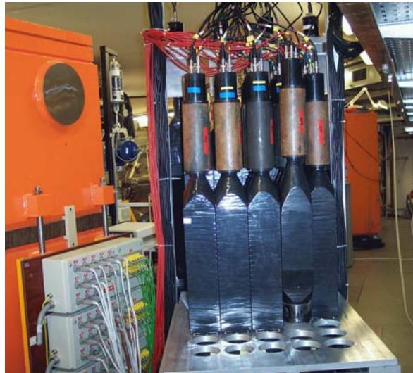
**Figure 2.11:** The detector for neutral particles at COSY-11.
