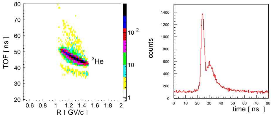
**Figure 3.4:** **Left:** Time-of-flight, measured on the path of 9.3 m between the scintillator hodoscopes S1 and S3, as a function of the magnetic rigidity. The figure shows only particles with an energy loss in the S1 scintillator larger than a value indicated by the dotted line in figure 3.3 (right). **Right:** Time of flight determined for the neutral particles between the target and the neutron detector.
