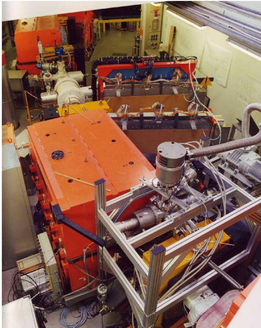
**Figure 2.2:** The COSY-11 detection system, showing the arrangement for the cluster target (bottom, right) the regular COSY dipole magnet (center, left) and the drift chambers and the scintillation detectors (top, right).
