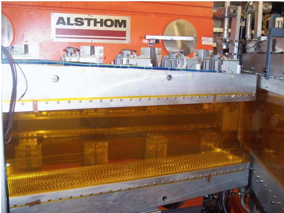
**Figure 2.7:** Drift chamber with a hexagonal cell structure in front of the COSY dipole.
