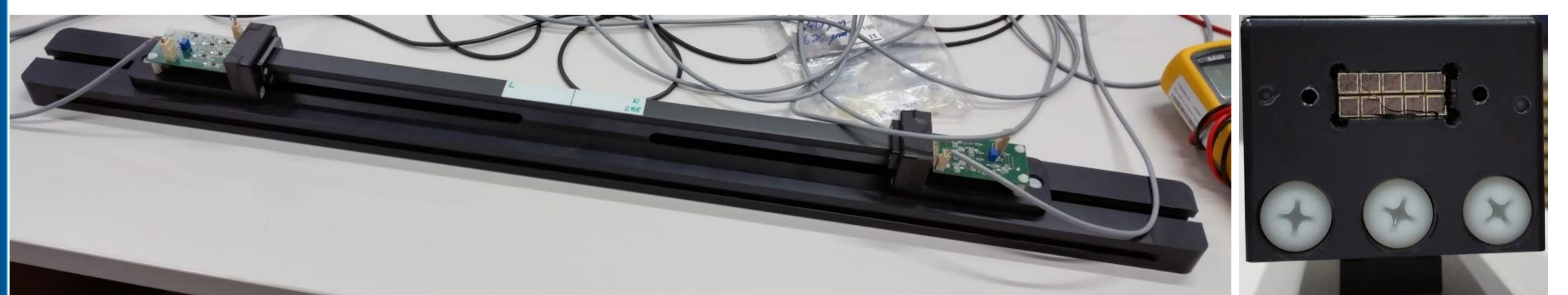
Fig. 7 (left) Photos of the prototype of novel J-PET detection module; scintillating stripe is wrapped in the black lightproof foil; (right) 2 x 5 Si-PM array with front-end boards attached from behind (green boards on left photo).
