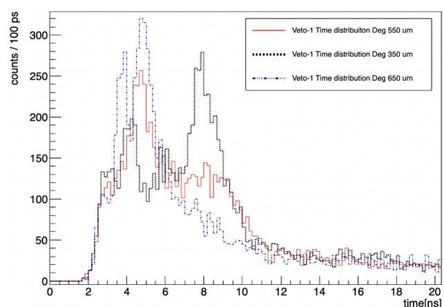
**Figure 4.** Veto-1 timing simulations for different degraders and the target filled with helium at 1.4% LHeD.
