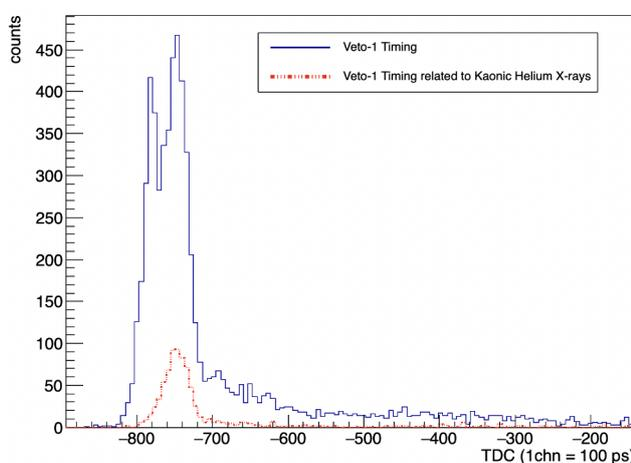
**Figure 3.** Veto-1 time distribution, in arbitrary unit of the Time to Digital Converter (TDC), measured during the SIDDHARTA-2 Kaonic Helium run. The red dotted line represents the time distribution of events related to kaonic Helium atoms.
