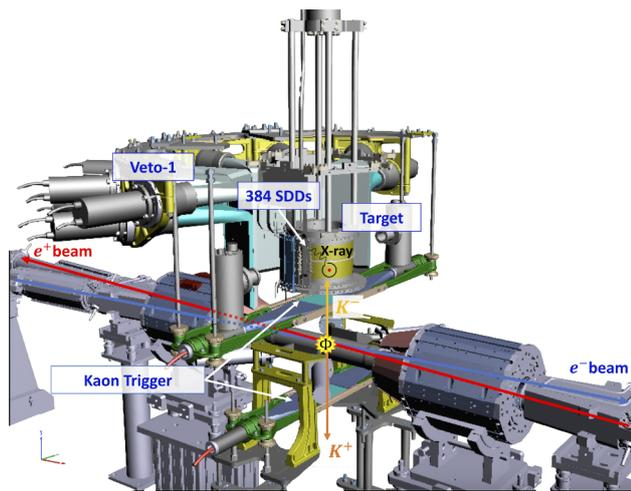
**Figure 1.** Schematic layout of the SIDDHARTA-2 experimental apparatus
