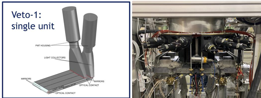
**Figure 2.** Left: Veto-1 single unit layout. Right: Photo of the Veto-1 system installed around the SIDDHARTA-2 vacuum chamber.
