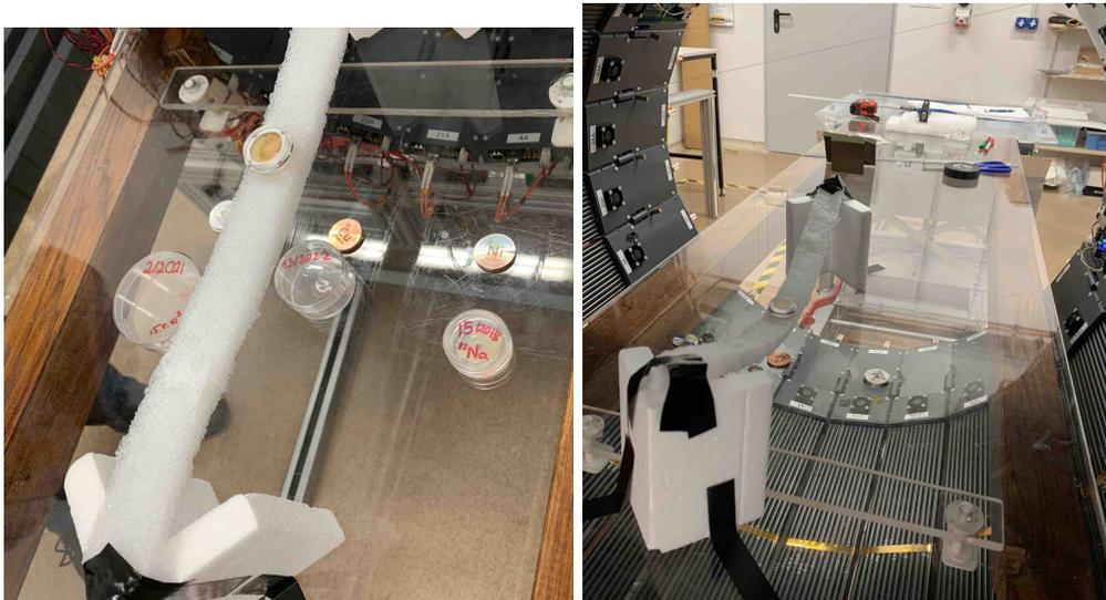
Figure 4.13: Placement of disks inside the J-PET modular scanner. *Left*: Before the start of the measurement. *Right*: The position of quartz in the  $y$  axis had changed during the measurement.
