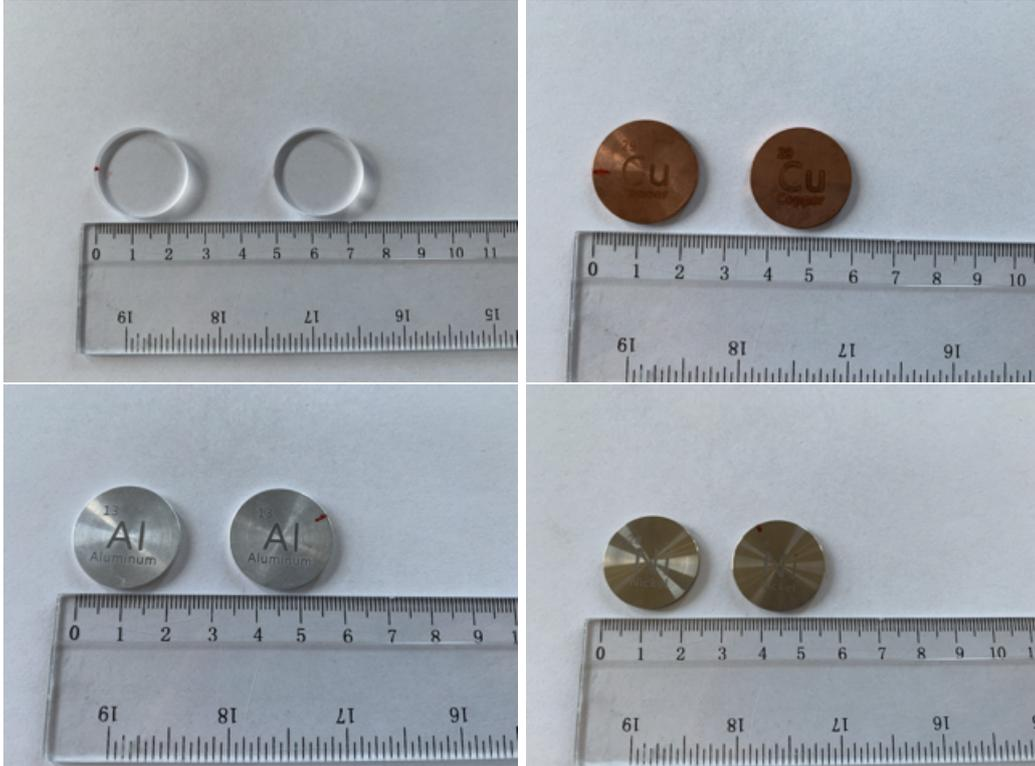
Figure 4.5: Pictures of the disks used in the study made of 4 different materials. *Top left to right:* Quartz and copper disks. *Bottom left to right:* Aluminum and nickel disks. The graduation scale of the caliper is 1 mm.
