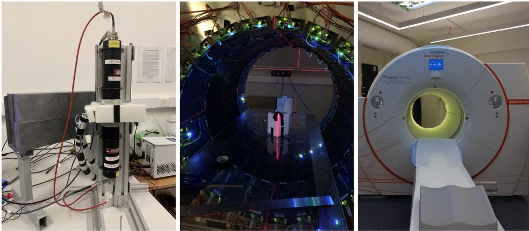
Figure 4.1: *Left:* The PALS setup in Jagiellonian University, Kraków. *Middle:* Modular J-PET scanner in Jagiellonian University, Kraków. *Right:* Biograph Vision Quadra PET/CT scanner in Inselspital in Bern, Switzerland.
