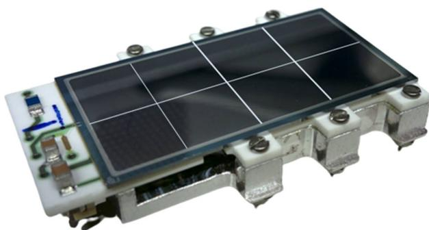
**Fig. 2** Silicon drift detector array for the SIDDHARTA-2 experiment with eight read-out cells indicated by the grey lines. The array is mounted on a ceramic carrier
