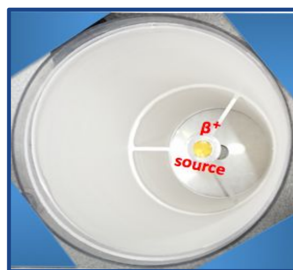
Fig.2 Pictorial representation of Annihilation chamber.
