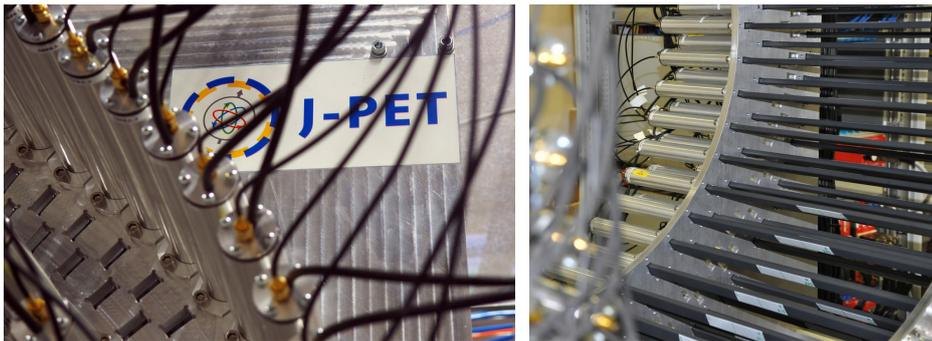
Figure 6.6: View of mounting plate with visible holes and photomultiplier tubes (left photo) as well as with scintillators (right photo). Courtesy of M. Glapska-Moskal and the J-PET group.
