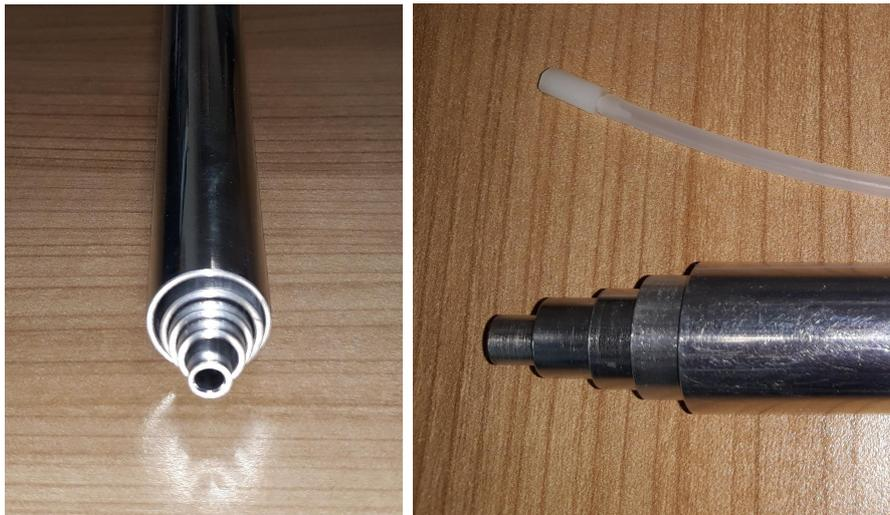
Figure 3.4: Sensitivity phantom with different tubes visible (left) and polyethylene tube (right).
