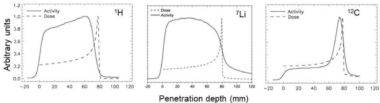
Figure 1. Depth distributions of calculated dose (dashed line) and measured  $\beta^+$ -activity (solid line) for  $^1\text{H}$  (left),  $^7\text{Li}$  (middle), and  $^{12}\text{C}$  (right) ions impinging in homogeneous targets of polymethyl methacrylate (PMMA,  $\text{C}_5\text{H}_8\text{O}_2$ ). (Adapted from references [4,5,6]). © Institute of Physics and Engineering in Medicine. Reproduced by permission of IOP Publishing. All rights reserved.
