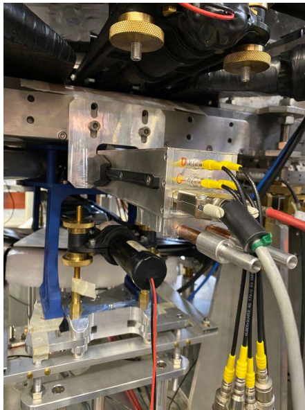
Figure 2: Photo of the aluminum box containing the four CZT detectors installed near the DAΦNE collider's beam pipe, during a test measurement.
