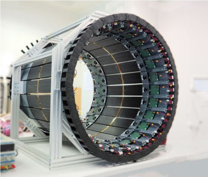
Fig. 2. The modular J-PET scanner prototype developed at Jagiellonian University. This modular architecture enables flexible configuration, high timing precision and efficient detection of photons.
