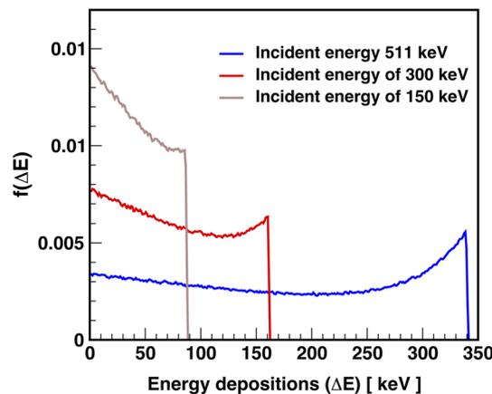
**Fig. 10** Normalized Klein–Nishina function describing the probability density distribution of energy depositions by photons of different incident energy in a plastic scintillator
