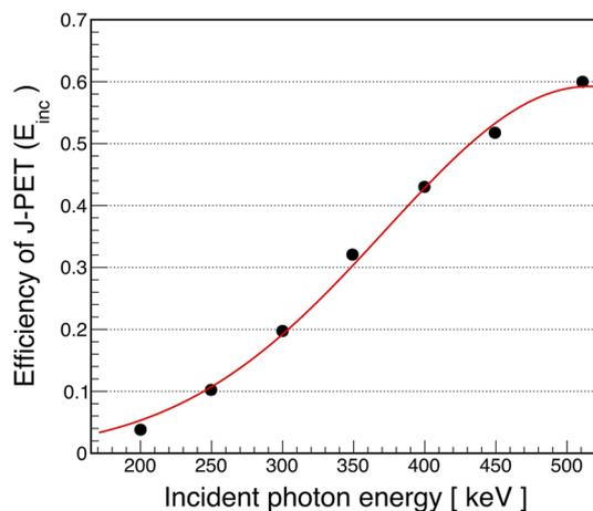
**Fig. 11** The intrinsic efficiency of the J-PET scanner as a function of the energy of the incident photon is shown by the black-filled circles. The red line shows the fitting function described in the text
