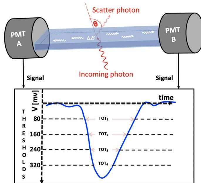
**Fig. 2** Illustration of deposition of energy by incident photons in the scintillator and obtaining the analog signal from both PMTs (A, B). The signals from each side are sampled at four equally spaced thresholds with minimum values of 80 mV and maximum values of 320 mV. The sum of  $TOT_i$ , where  $i$  is the number of thresholds, gives the measure of energy deposition calculated by Eq. 1
