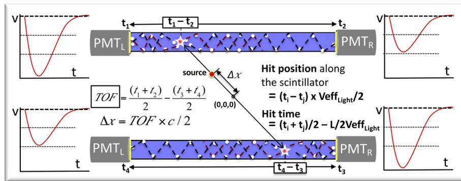
**Fig. 3** Demonstrates the principle of the J-PET scanner based on two plastic strips. Analog signals measured at four PMTs are also shown. For a scintillator of length L and considering the effective velocity of the light photons inside the scintillator (V<sub>eff,Light</sub>), the formula for calculating the hit position and hit time is shown in the figure. The annihilation point can be reconstructed from the measured TOF information between two hit positions (in different/opposite stripes)
