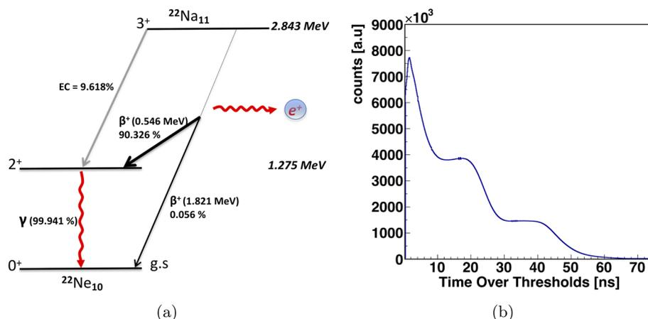
**Fig. 5** **a** Shows the decay scheme of the  $^{22}\text{Na}$  source. **b** shows the typical TOT spectrum for the  $^{22}\text{Na}$  source determined for events with 3 registered hits. The detailed description of the spectrum can be found in the text
