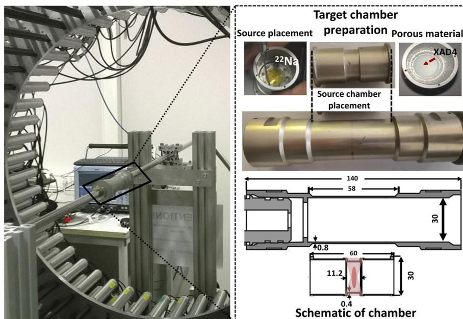
**Fig. 4** Left panel shows the experimental setup. The source chamber was aligned in the center of the J-PET tomograph. The upper part of the right panel shows the zoomed version of the source chamber and its preparation. The bottom part describes the schematic of the target chamber with dimensions (in mm). The red color in the center of the small cylinder represents the position of the source
