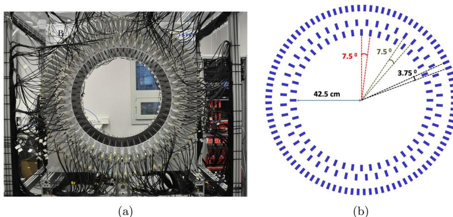
**Fig. 1** **a** Front view of the 192 modules prototype of J-PET scanner (see text for description). **b** Shows the cross section of J-PET with azimuthal angular displacement of the scintillators arranged in 3 layers
