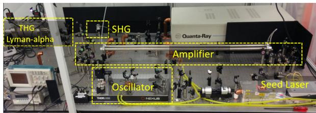
Figure 5: The ATRAP pulsed Lyman alpha (121 nm) system that is now operating in the ATRAP laser cabin.
