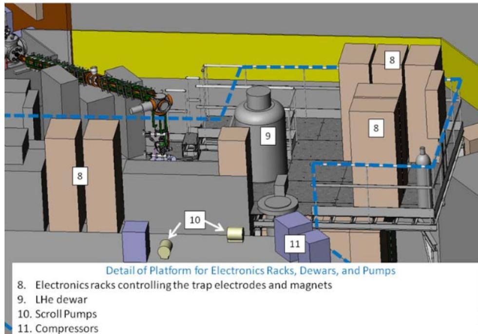
Figure 11: The antihydrogen production area (ATRAP zone 2) includes a platform on which supporting electronics and cryogen dewars are stored.
