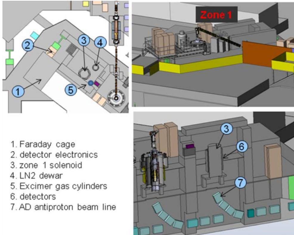
Figure 9: Precise comparisons of antiprotons and protons take place in ATRAP zone 1.
