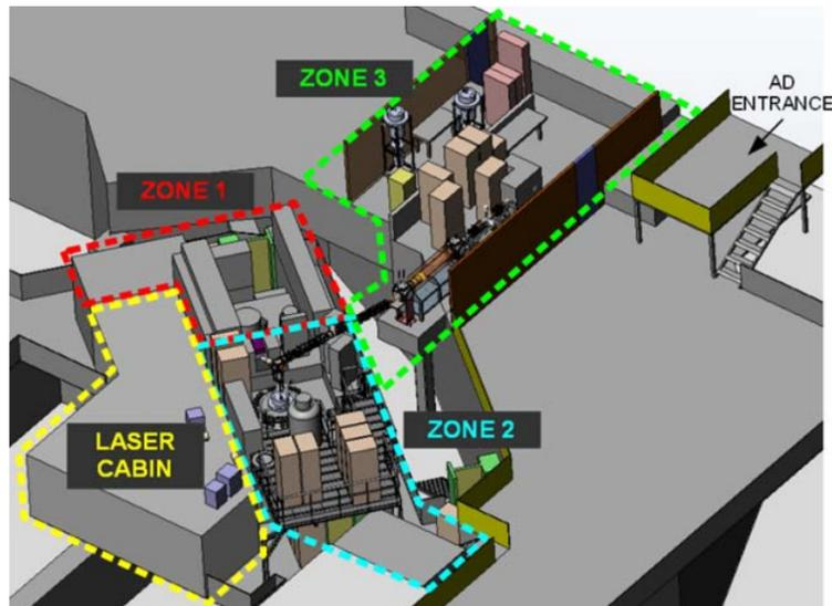
Figure 8: Top representation of the three ATRAP experimental areas. Antiprotons are available for precise antiproton experiments (zone 1) and for antihydrogen experiments (zone 2). The positrons needed to make antihydrogen are produced in third area (zone 3).
