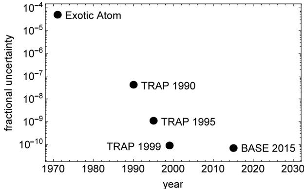
Figure 4: The 1999 comparison of the charge-to-mass ratios of the antiproton and proton performed by TRAP [15] was confirmed in 2015 by BASE [27] at essentially the same uncertainty. (The quoted uncertainties were about 20% smaller.).
