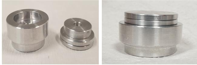
Figure 9.7: Aluminium chambers for measuring PALS in spheroid samples.
