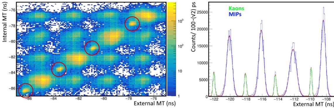
**Fig. 2** Left: 2-D plot of the TDCs coincidence between the internal ( $(TDC1+TDC4)/2$ ) and external ( $(TDC2,TDC3)/2$ ) luminosity monitor scintillators. Red circles indicate the kaons distribution; Right: Projection on the time coordinate of the 2D plot diagonal
