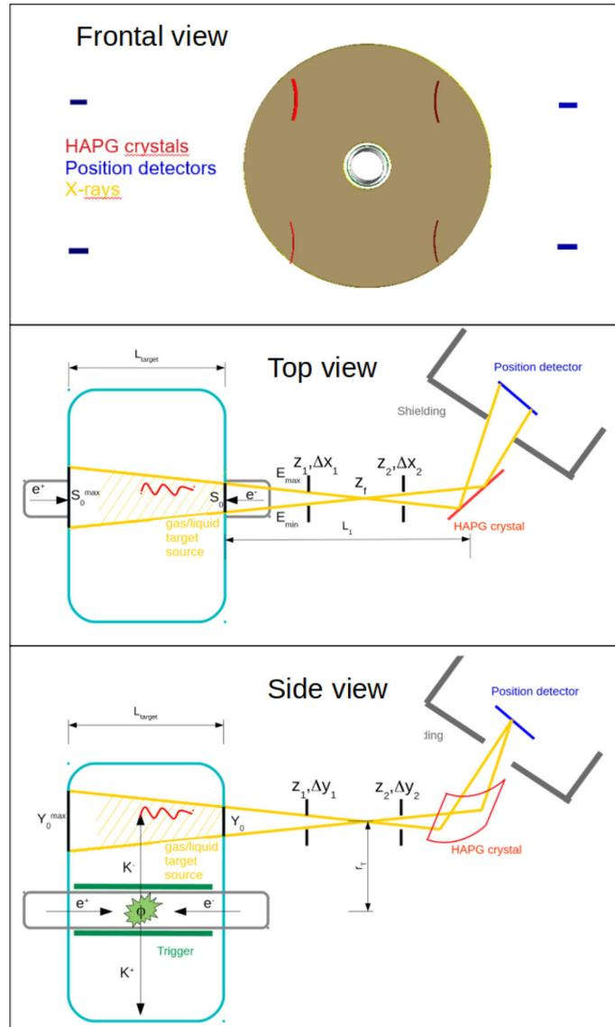
**Fig. 5** Sketch of a possible setup of the KA3 experiment (see text for details)
