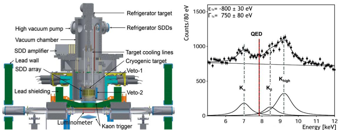
**Fig. 1** Left: Cross section layout of the SIDDHARTA-2 experimental apparatus (red dot box refers to the SIDDHARTA-2 luminometer). Right:  $K^-d$  MC simulation for an integrated luminosity of 800 pb<sup>-1</sup> considering  $\varepsilon_{1s} = -800$  eV,  $\Gamma_{1s} = 750$  eV and yield=0.1% as input parameters
